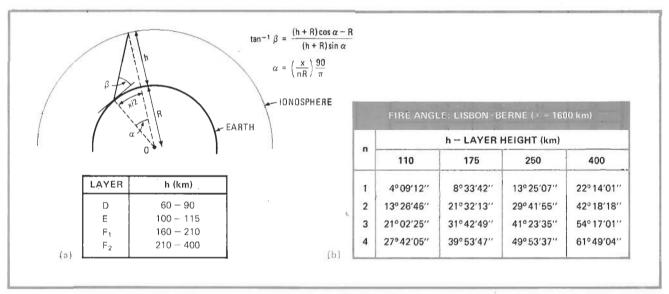
**lonospheric propagation.** Antenna's firing-angle equation is derived from simple geometric considerations and yields fairly accurate results (a). Vertical angle of radiation required is tabulated versus layer height and hop number for the path separating Lisbon and Berne (b).
